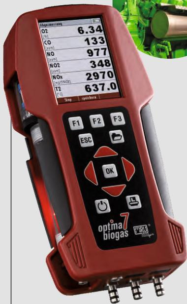
Professional handheld analyser with all combustion and emission calculations and automatic measurement incl. data logging function, configurable by user.
