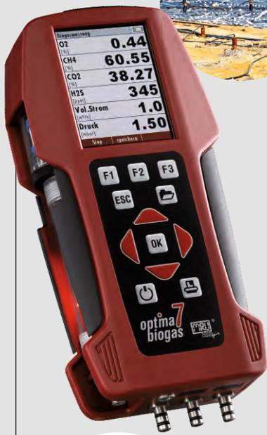
Professional handheld analyser using a special 3-components-gas sampling probe, designed for the use at landfill sites.
